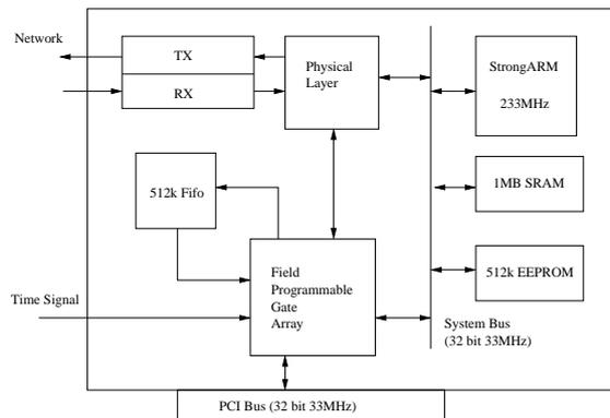
Fig. 2. Dag hardware measurement card
